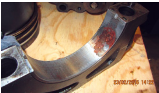
Figure 26: Water contamination of the lubrication oil caused cavitation damage on a crankshaft bearing; source: VGH
