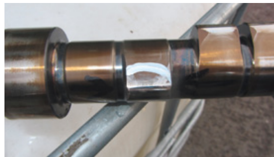
Figure 22: Defective plunger; source: VGH
