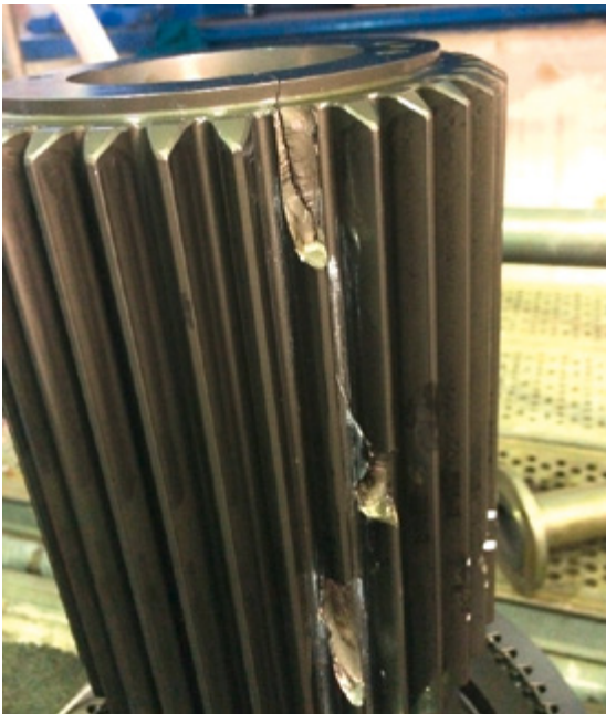
Figure 6: Torn sun pinion with broken teeth; source: Teko
