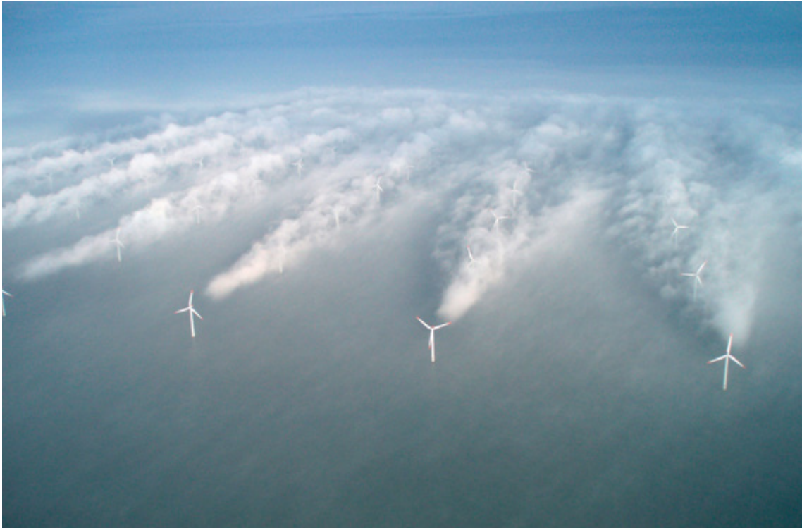
Figure 60: Wake effect due to turbulent air flow at the wind park Horns Rev 1; source: Vattenfall
