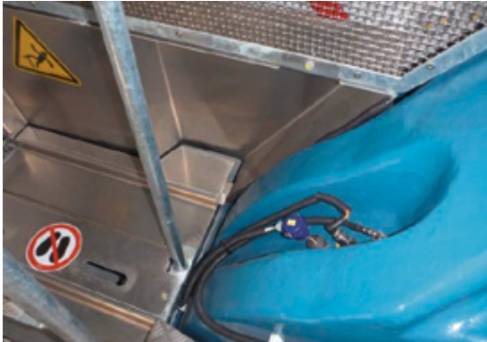
Figure 24: Sensor on the main bearing. It is designed to detect damage caused by the slowly rotating shaft. Bearing vibrations can arise in the low-frequency range below 10 Hz.
