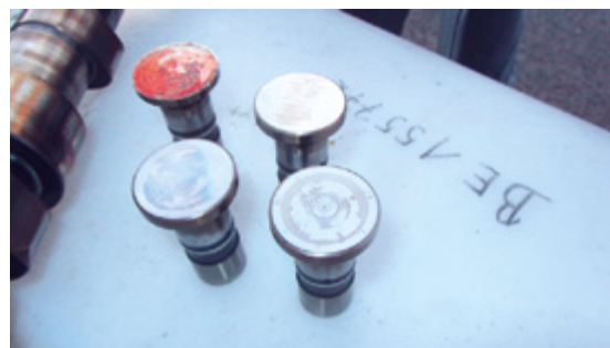
Figure 23: Due to a defective plunger, the camshaft had to be replaced, source: VGH
