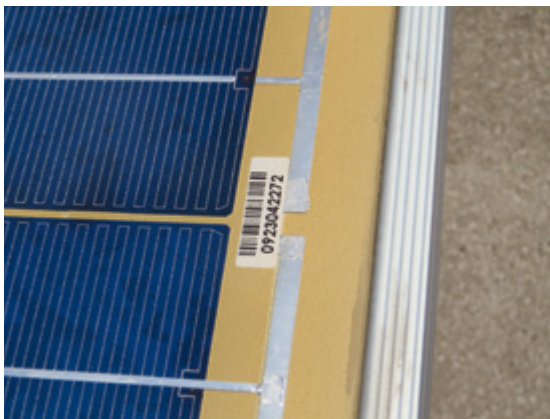
Figure 2: Yellowing of the film on the back of a PV module. In the long term this discolouration leads to a reduction in performance; source: PVGutachten.info
