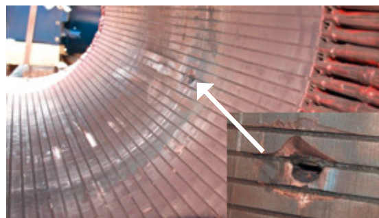
Figure 40: Generator-stator winding with earthing; source: R+V
