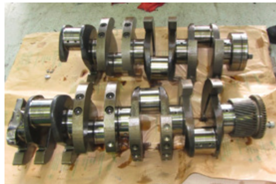
Figure 20: This crankshaft broke after 5,000 operating hours; source: VGH
