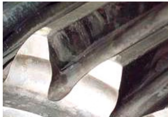
Figure 34: Grey stains on the sides of gear teeth; source: Allianz
