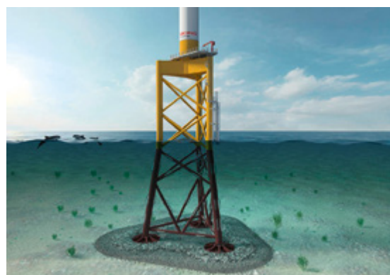
Figures 51–52: Jacket structure on suction buckets; source: DONG Energy
