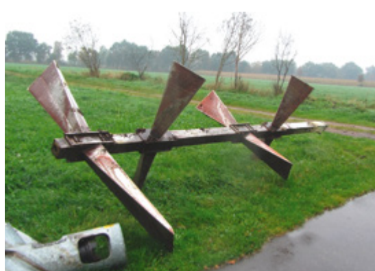
Figure 8: A fractured agitator; source: VGH
