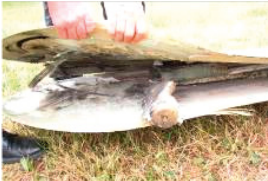
Figure 28: Broken blade tip after lightning strike; source: Allianz
