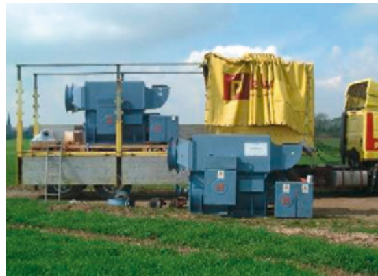
Figure 16: Double-fed asynchronous generators for on-site installation; source: Allianz
