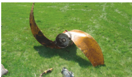
Figure 6: Torn propeller; source: VGH
