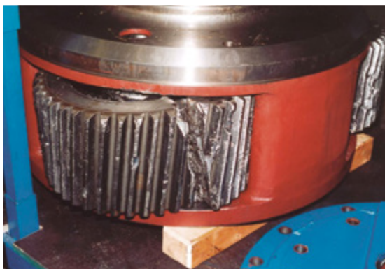
Figure 33: Total damage of the transmission after bearing failure at the planetary carrier after approximately 20,000 operating hours (1 MW wind turbine); source: Allianz
