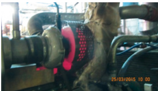
Figures 30–31: Turbocharger, ~600 °C; source: VGH
