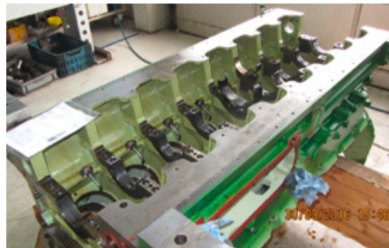
Figure 21: Consequential damage to the engine block; source: VGH
