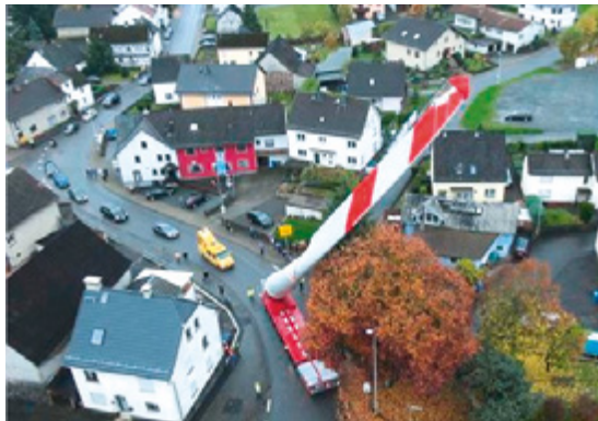
Figure 12: Rotor blade transport with a blade transport vehicle, Goldhofer AG; source: Goldhofer AG
